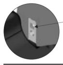
NOTE: Use square hole, not round hole, when assembling plinth to legs.
